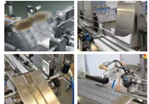
High rate reject systems
